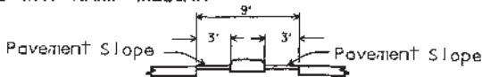
FIGURE 2.25 Cross-section information for interchange elements—pavement, shoulders, and medians. (From Location and Design Manual, Vol. 1, Roadway Design, Ohio Department of Transportation, with permission)
